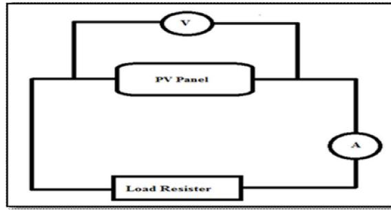
**Figure 1: PV panel test circuit Schematic diagram**
