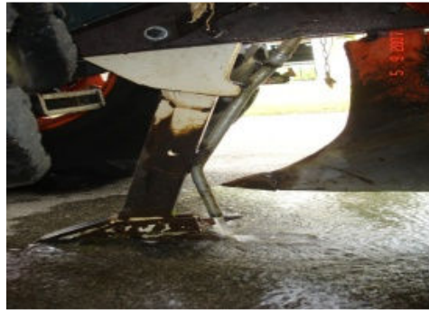
(a) Subsoiling and liquid Fertilizer Tube
