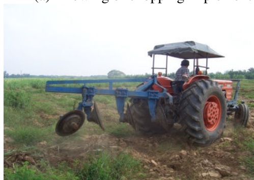
(b) Three disc plow for conventional land preparation
