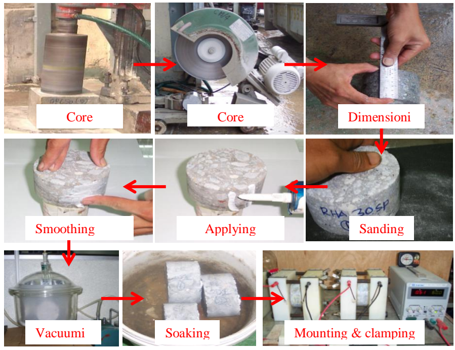
Figure 7: Steps involved in the preparation of the specimen before conducting the RCPT
