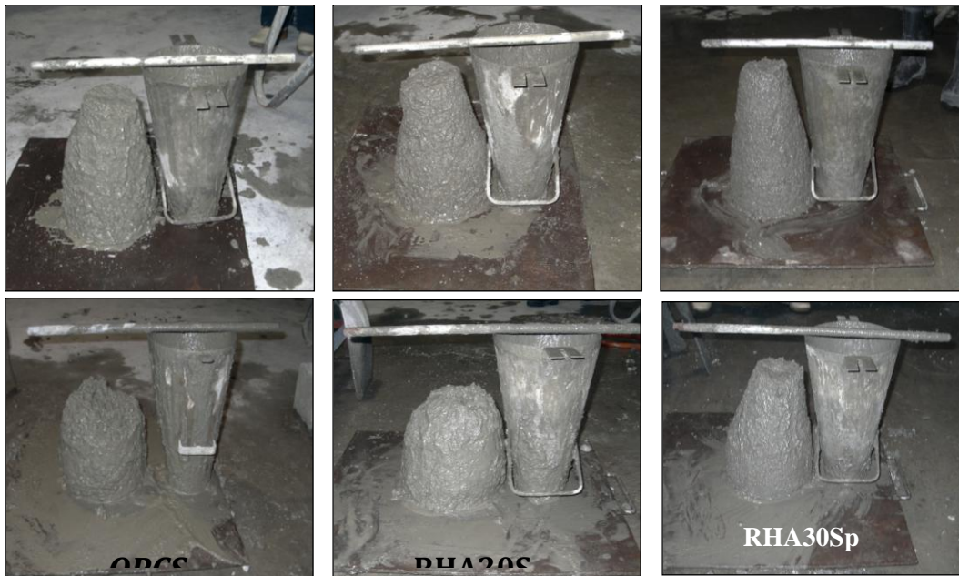
Figure 3: The slump for the various mixes of fresh concrete with and without Sp
