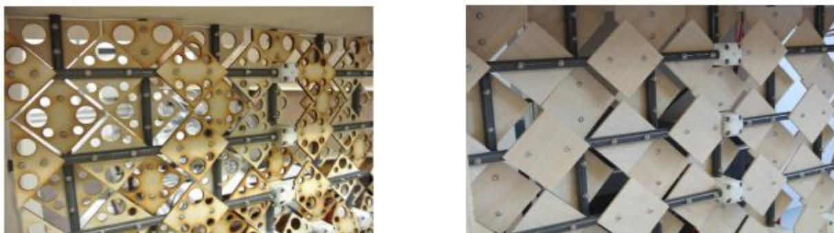
Figure 11: Cutout Wings, TEST CASE 1 (left) and Solid Wings, TEST CASE 2 (Right) 5 .
