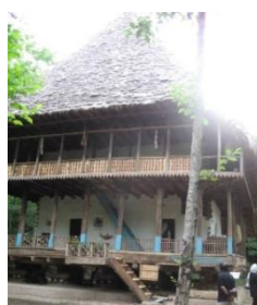
Figure 5. High slope of roofs in order to protect buildings from the rain and snow
