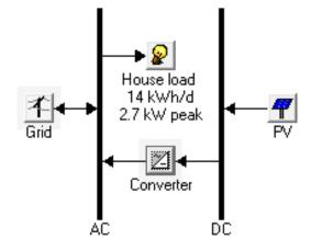
Figure 5: system configuration.
