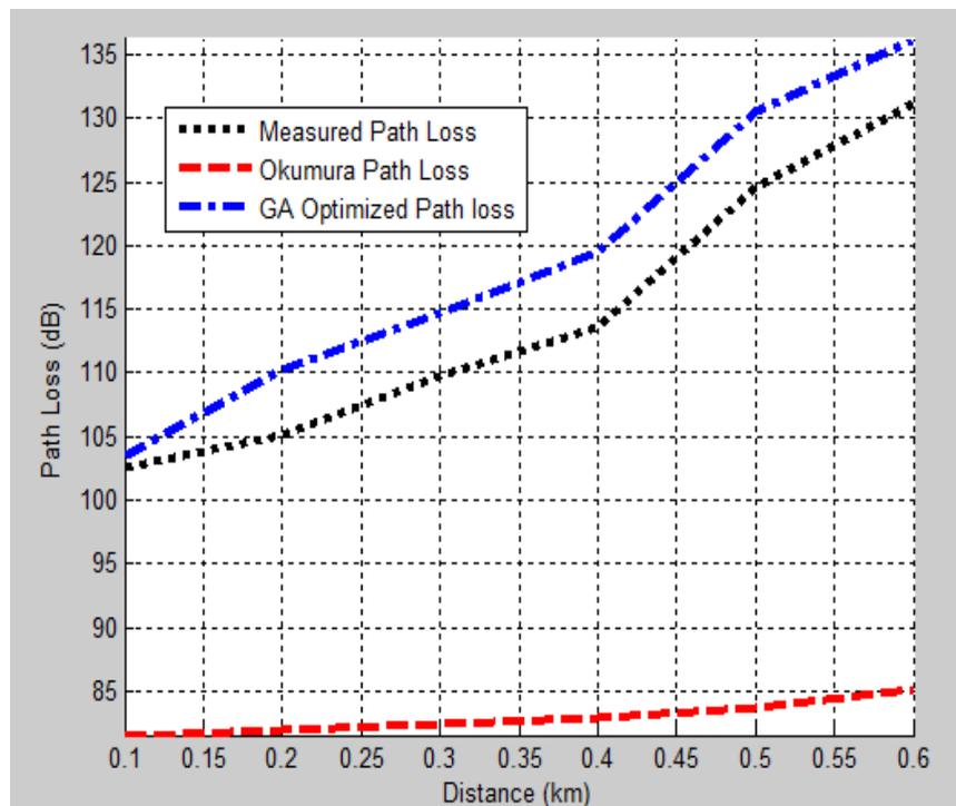
Figure 6: Pathloss of the measured, GA optimized, and Okumura-Hata model values versus distance for the LTE base station 4
