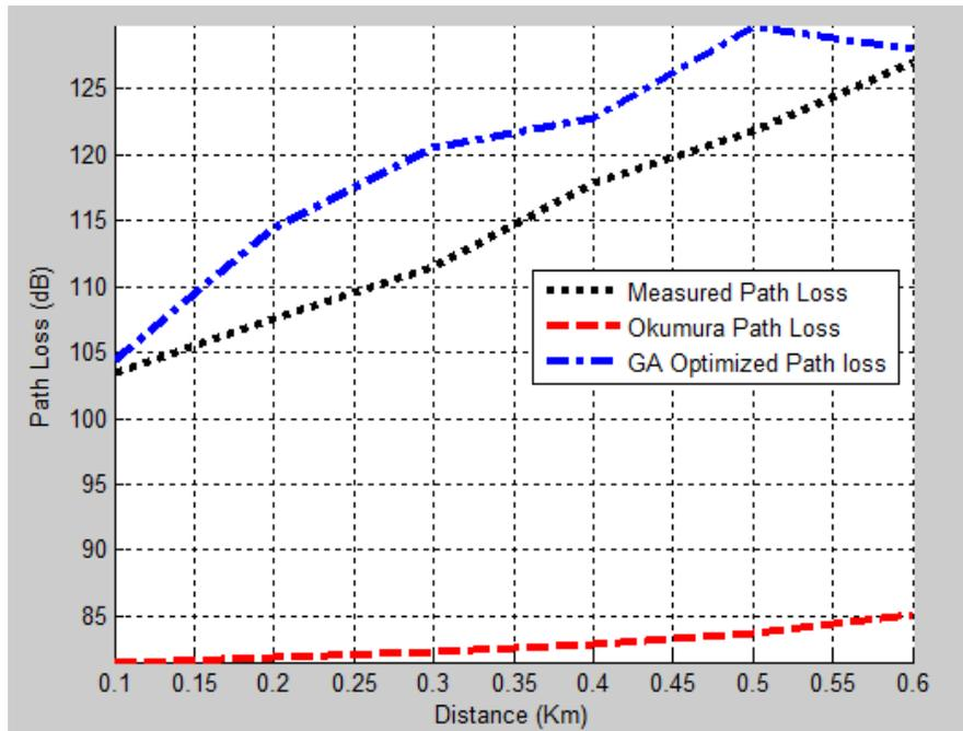
Figure 3: Pathloss of the measured, GA optimized, and Okumura-Hata model values versus distance for the LTE base station 1
