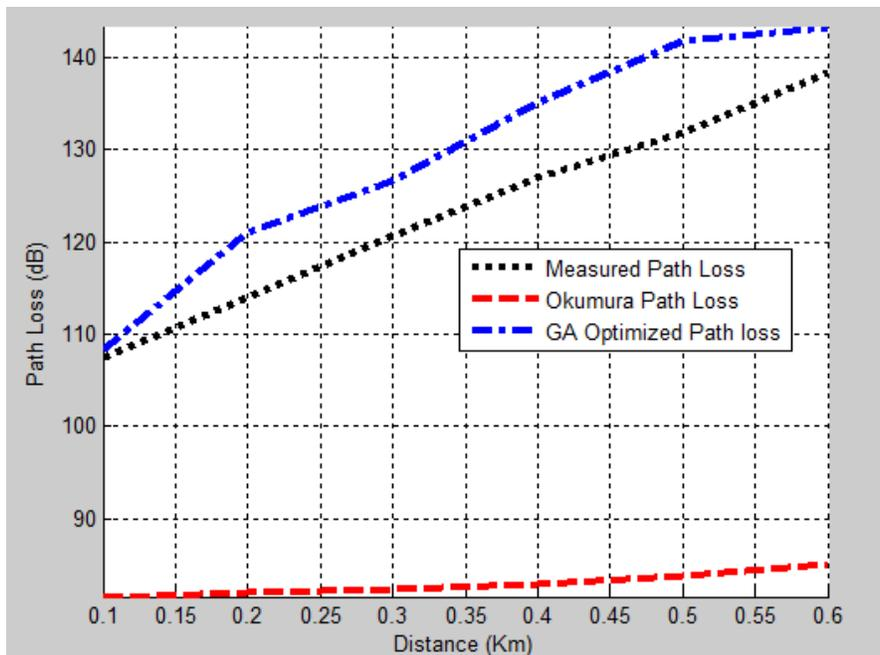
Figure 4: Pathloss of the measured, GA optimized, and Okumura-Hata model values versus distance for the LTE base station 2
