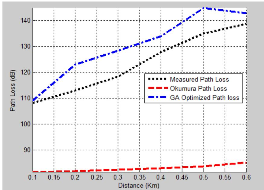
Figure 5: Pathloss of the measured, GA optimized, and Okumura-Hata model values versus distance for the LTE base station 3
