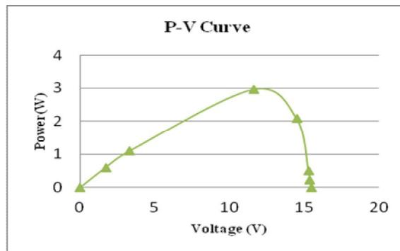
**Figure 3: P-V Curve for Monocrystalline PV panel**
