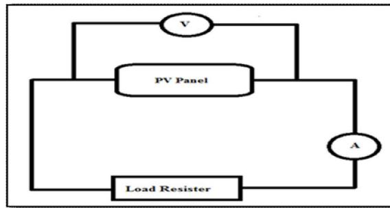
**Figure 1: PV panel test circuit Schematic diagram**
