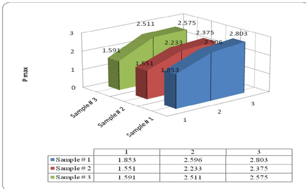
**Figure 4: 3D Graph for the Pmax with Different Dust Mass Density for the Research Samples**
