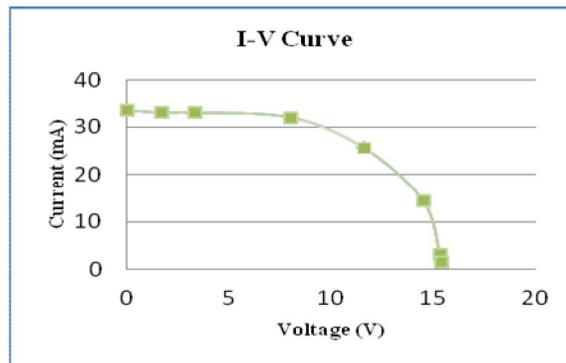
**Figure 2: I-V Curve for Monocrystalline PV panel**
