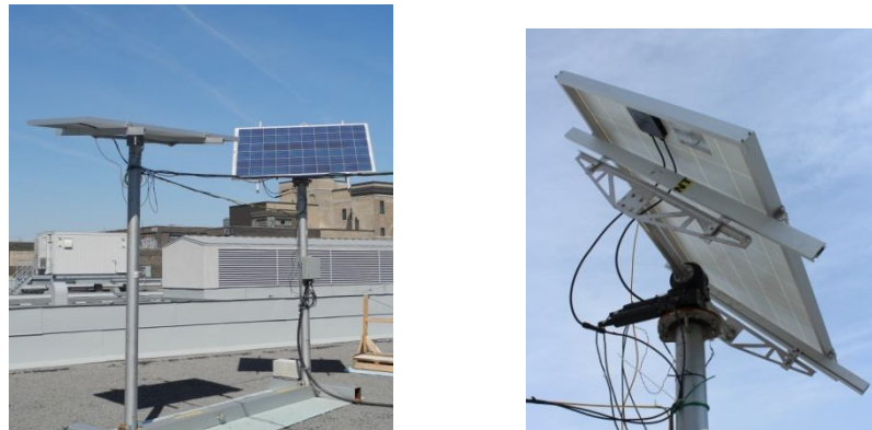
Fig.1: Picture of the experimental set up : (left) overview of both PV panels with the fixed and horizontal panel on the left and the solar tracking panel on the right ; (right) close-up of the motors of solar tracker
