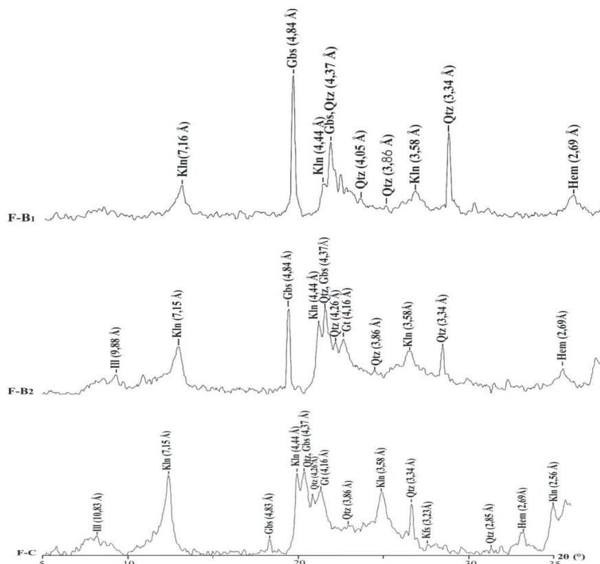
Figure 3: XRD Patterns of Mineral Constituents of Loose Weathered Materials on Trachyte
