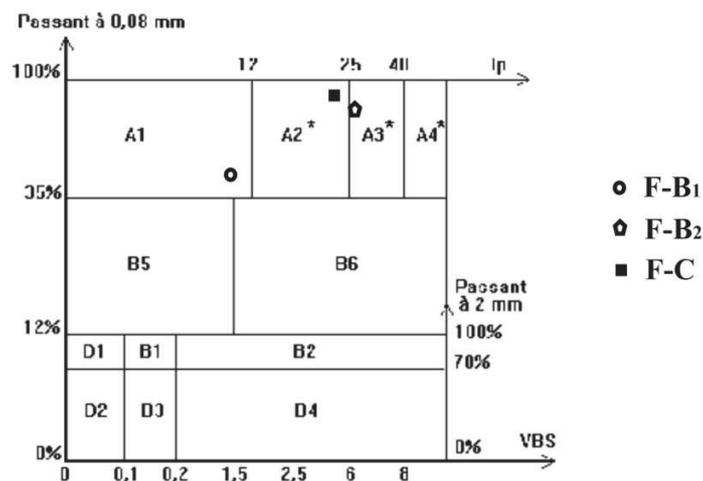
**Figure 7 : Classification of loose weathered trachyte to according to Guide de Terrassement Routier (GTR)**
