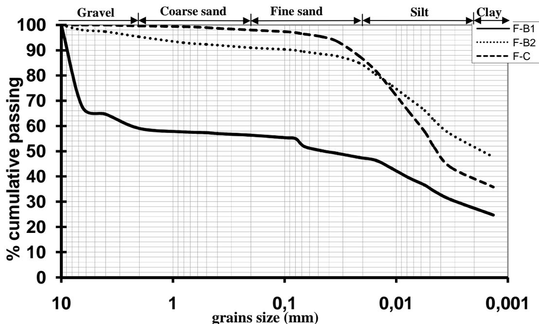
Figure 4 : Granulometric curves of Loose Weathered Materials on Trachyte
