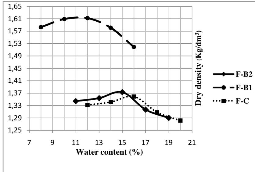
Figure 5: Compaction Test Curves of Loose Weathered Materials on Trachyte
