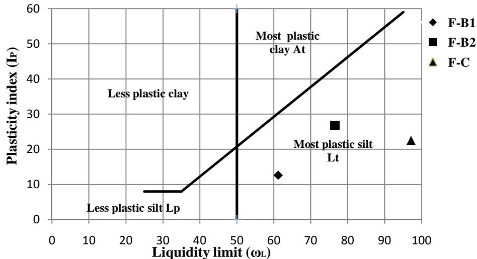
**Figure 6 : Classification of Loose Weathered Materials on Trachyte According to the Laboratoire Central Des Ponts et Chaussées (LCPC)**
