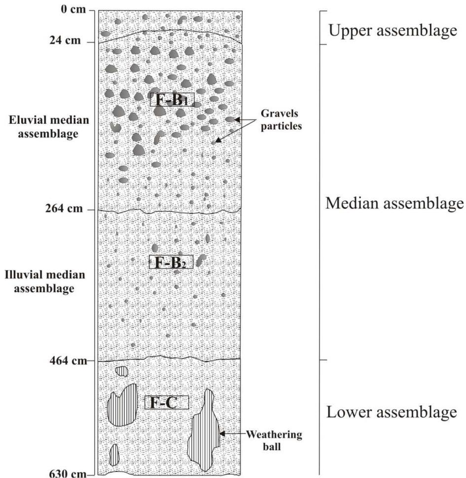
**Figure 2: Weathered Soil Profile on Trachyte**
