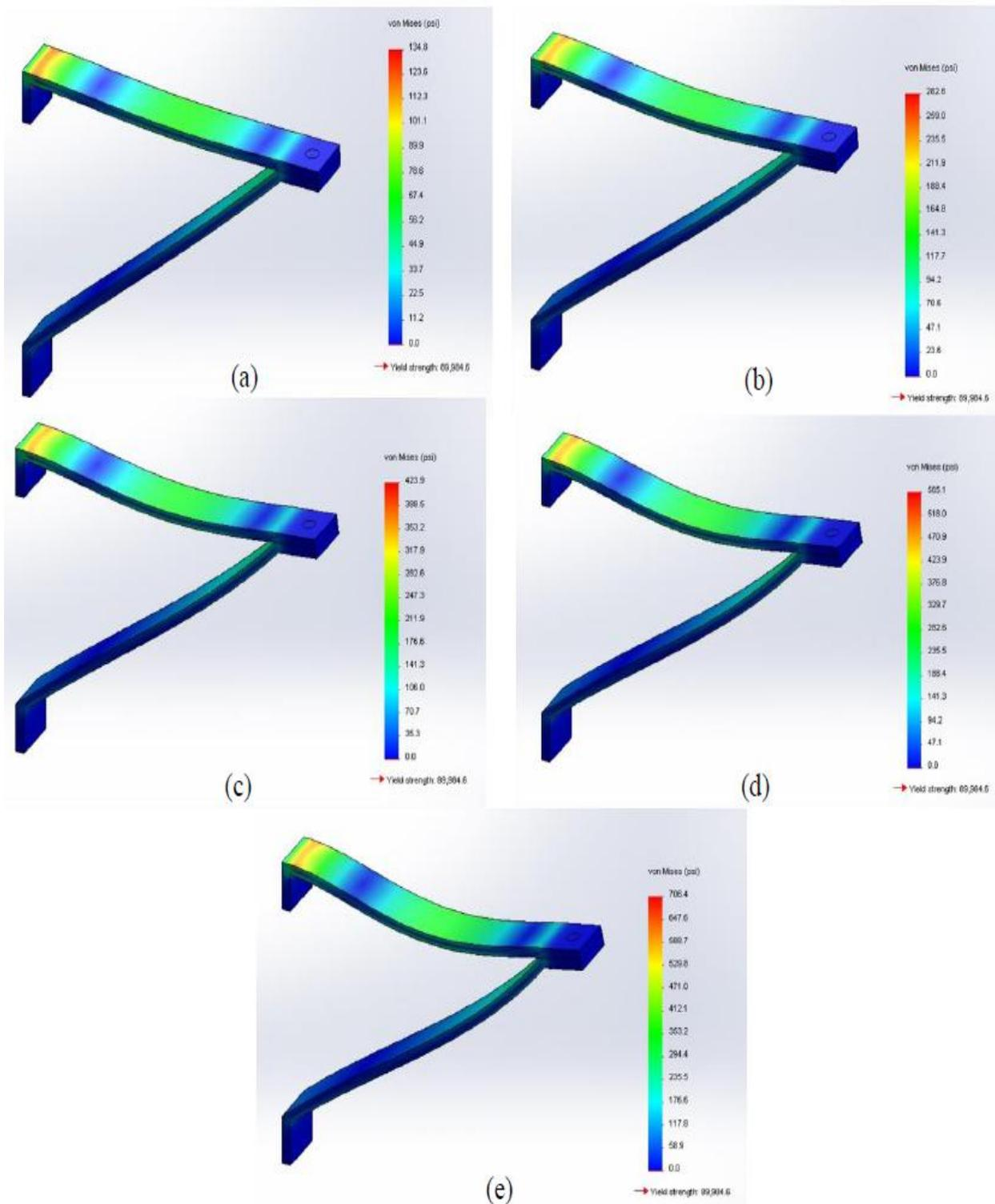
Fig. 5: Von Mises Stress (in psi) Plots for (a) 10 lbs, (b) 20 lbs, (c) 30 lbs, (d) 40 lbs, and (e) 50 lbs
