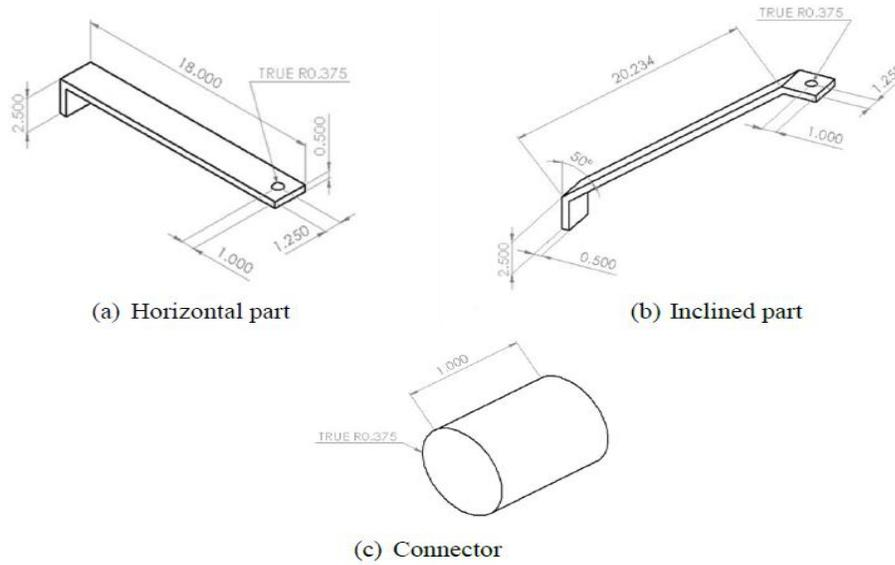
**Fig. 3: Dimensions (in inch) of the Hanger Components**
