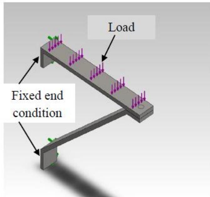
**Fig. 4: Simulation of Load and End Conditions**
