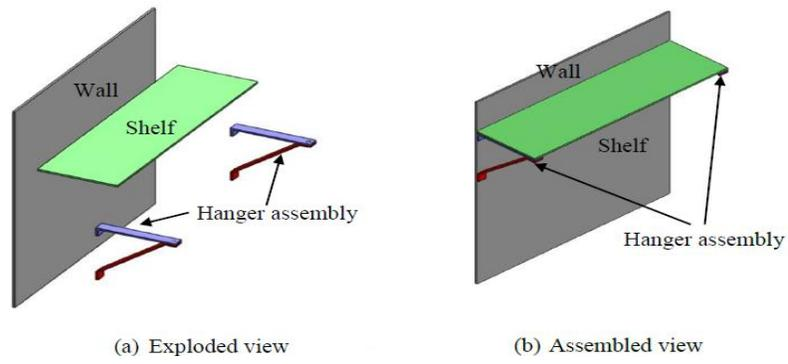
**Fig. 2: Two Hanger Assemblies Attached to a Wall and Supporting a Shelf**
