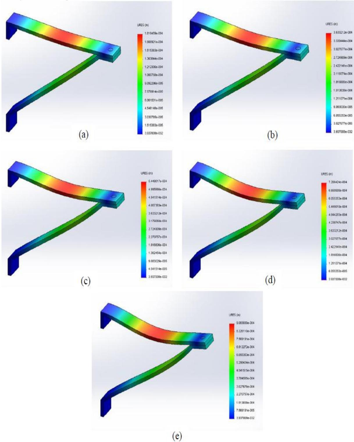
Fig. 6: Displacement Plots (in inch) for (a) 10 lbs, (b) 20 lbs, (c) 30 lbs, (d) 40 lbs, and (e) 50 lbs
