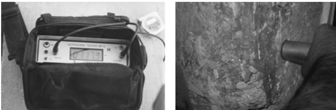
**Figure 1: Ultrasonic Velocity Test, with an “Ultrasonic Tester”, on a Concrete Reinforced Element Under Investigation**
