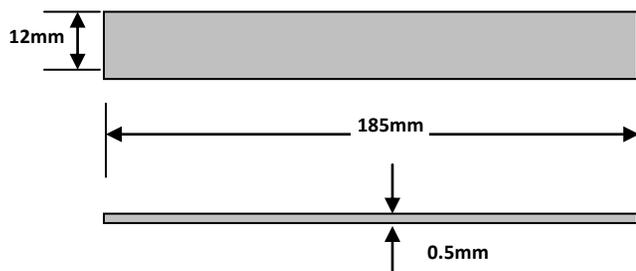
Fig.2.The dimensions of stainless steel sample.
