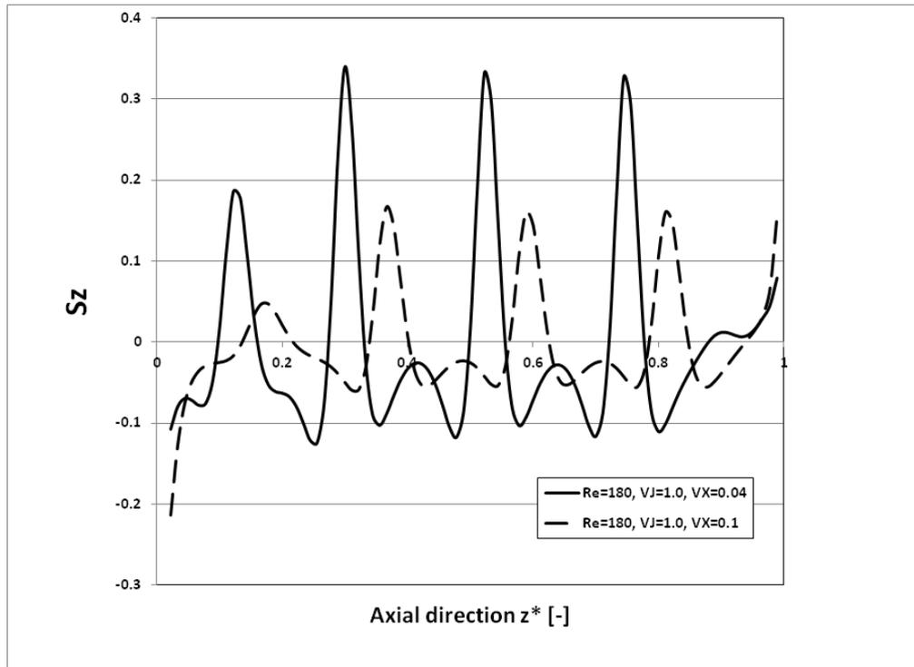
Fig. 7. Effect of the axial return flow intensity on the evolution of the axial component of the shear rate near the borehole wall for  $VX=0.04$  and  $VX=0.1$  ( $Re_{rot}=180$ ,  $VJ=0.1$ ).
