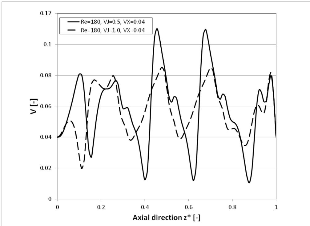
Fig. 5. Effect of jet intensity on the axial velocity at the middle of the annulus for values of  $VJ=1.0$  and  $VJ=0.5$  ( $Re_{rot}=180, VX=0.04$ )
