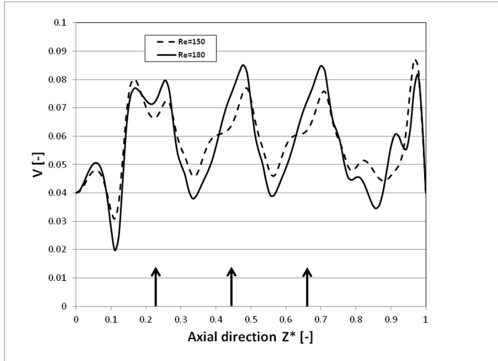
Fig. 3.Axial velocity evolution at the middle of the annulus for  $Re_{rot}=150$  and  $Re_{rot}=180$  ( $VJ=1.0$  and  $VX=0.04$ )
