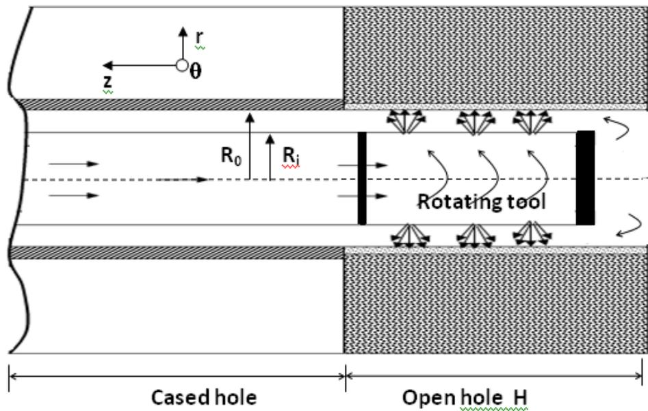
Fig. 1. Schematics of the set-up arrangement.
