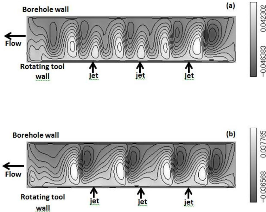
Fig. 4. Iso-contours of the flow streamlines.
