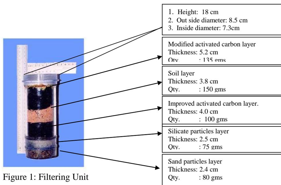
Figure 1: Filtering Unit
