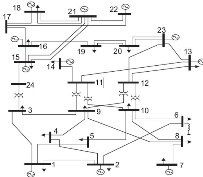
Figure 2. IEEE 24-bus test system
