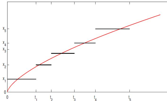
Figure 1: Step and varying stress accelerated life tests.
