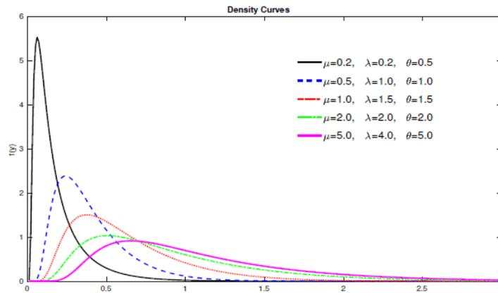
Figure 2: TIG ( $\mu, \lambda, \theta$ ) density curves for various parameter values.
