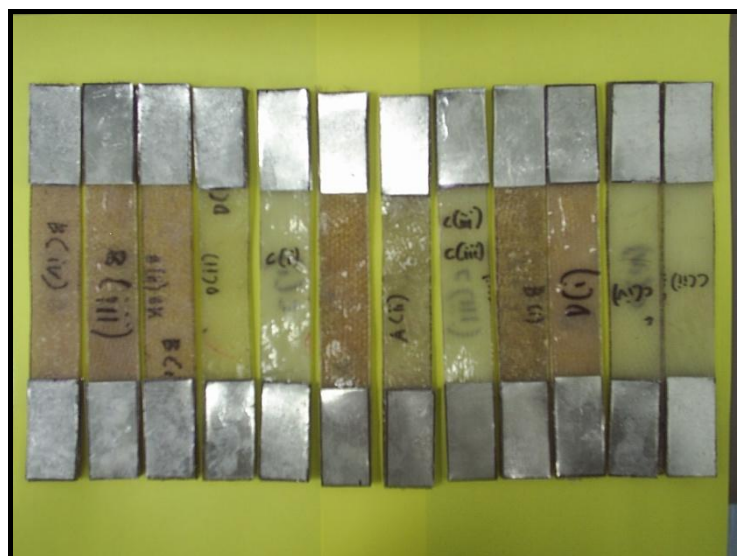
Figure 1: Specimen for tensile test ASTM D 3039
